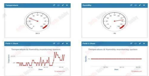
Gambar 4. Hasil Data Pengujian sensor suhu (DHT11) di Web thingspeak
