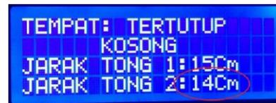
Gambar 13: Tampilan LCD Jarak Tong 2
