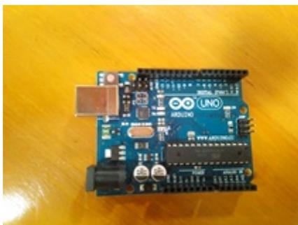
Gambar 1: Mikrokontroler Arduino UNO R3
