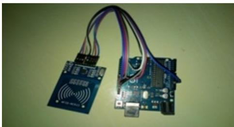
Gambar 9: Rangkaian RFID Arduino
