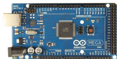
Gambar 3: Board Arduino Mega 2560
